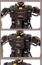
RoboPhilo comes with a powerful robot controller with 24 servo channels and up to 8 I/O interface. A specialized interrupt driven kernel is used to handle motion and remote controls on demand. RoboPhilo is readily programmable directly from your PC to design and perform your personalized movements. This robot is developed to attract more entry-level hobbyist and students looking for hands on experience with robotics building and programming.
